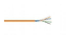
Kramer's BCLS-33 is a high-performance CAT 6A F/UTP cable designed for IT, LAN and Ethernet installations. It is constructed with 23AWG solid bare copper conductors with a cross filler and overall metal foil screen with a drain wire. It is enclosed in an LSZH jacket with sequential markings every meter and packed on a fumigated plywood reel. BCLS-33 cable exceeds CAT 6A specifications to provide additional performance and bandwidth beyond the basic standard
